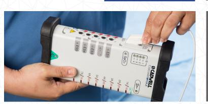
Mount Modules to the OR table with rail brackets and clamps. Easily insert and remove electrodes with the Quick Adapt.
